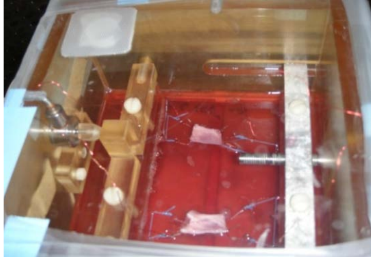
Figure 5.1 Tissue culture chamber showed the tissue constructs mounted onto the fixed arm and the movable arm
